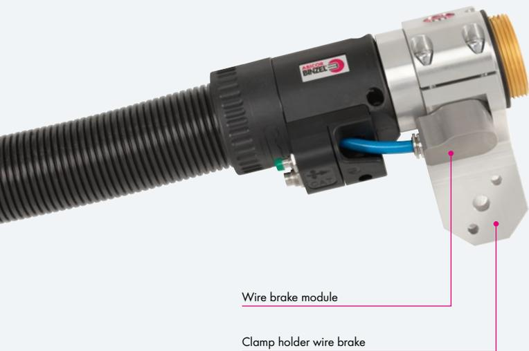
For tactile component search using the established ABIROB® W cable assembly, cable assemblies can now come with an optional wire clamp function to fix the wire. This function enables locking the wire in the cable assembly via a pneumatically operated piston that pushes the wire against an abutment. This ensures that the wire remains in position during sensing.
